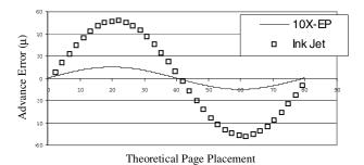
Figure 1, Relative advance errors of a feed roll with 300 microns amplitude error and 0 bias placed in a 600 DPI Electrophotographic system (shown at 10 times the error) and a 600 DPI Ink Jet system printing in two passes
