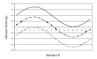
Figure 2. The effects of bias on the paper advance error.
