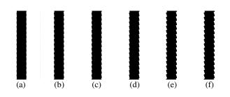
Figure 4, Line Edge Quality of Lines Parallel to the Advance Direction (here rotated 90degrees). Simulated 600 DPI printer using a 3 inch diameter feed roll and (a) 100, (b) 200, (c) 250, (d) 300, (e) 400 and (f) 500 micron error amplitude.
