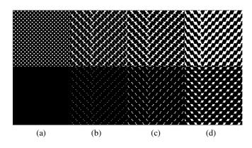
Figure 3. 50% Checkerboard Pattern Quality (rotated 90 degrees). Simulated micrographs. The top row printed with a 60 $\mu$  while the bottom used an 80 $\mu$  spot. (a) Perfect, (b) three inch roll diameter, (c) two inch roll diameter and (d) one inch roll diameter all having 300  $\mu$  sinusoidal amplitude error on the radii
